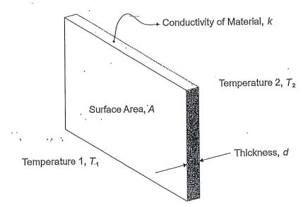
The rate at which heat is conducted through a material depends on temperature (K) on both sides of the material ( $T_1$  and  $T_2$ ), the surface area A ( $m^2$ ) exposed, the thickness of the material d (m) and the property of the material known as conductivity k.
